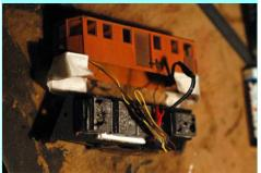
GOO the lamps to the body, tidy up the wires with some tape, plug the connector together for the trolley pole and your ready to close up the model. There is really not Front or Back for the model, but I did set it up so the model would run with the large door on the curb side when running on street trackage with the controller set to Forward.
